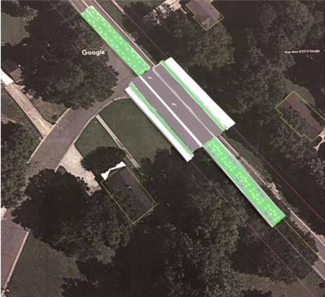
Group 2's plan had a 10' MUP on the north, a 5' sidewalk on the south and 4' planting strips on both sides of the street. This plans had one 11' travel lane going in each direction and a left turn
