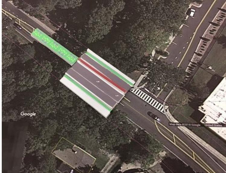
Group 1's plan for this section had 4' planting strips on both sides of the street, a 10' multi-use path (MUP) on the south side of the street and a 5' sidewalk on the north side of the street. Traveling east was an 11' travel lane and 23' planted median that changed to a left turn lane and 6' median onto Charles Buckley Way. Traveling west was an 11' travel lane.
