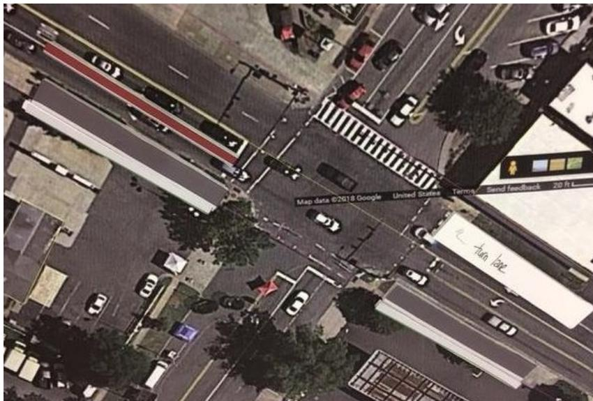
Group 2 took the existing street cross section and added an eastbound through lane and, on the west side of the intersection, a 4' median that would restrict vehicles from entering the left turn
