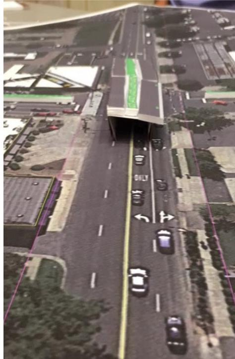
Group 3's plan was more conceptual in nature called for a bypass tunnel where travelers planning to pass through and not stop in Matthews would pass under downtown via a tunnel. The at-grade section (on top of the tunnel) contains an 11' eastbound travel lane and a 14' westbound shared travel lane (cars and bikes) separated by an 8' planted median. The tunnel aspect of this road section is so conceptually different that it makes comparison with the other sections difficult.
