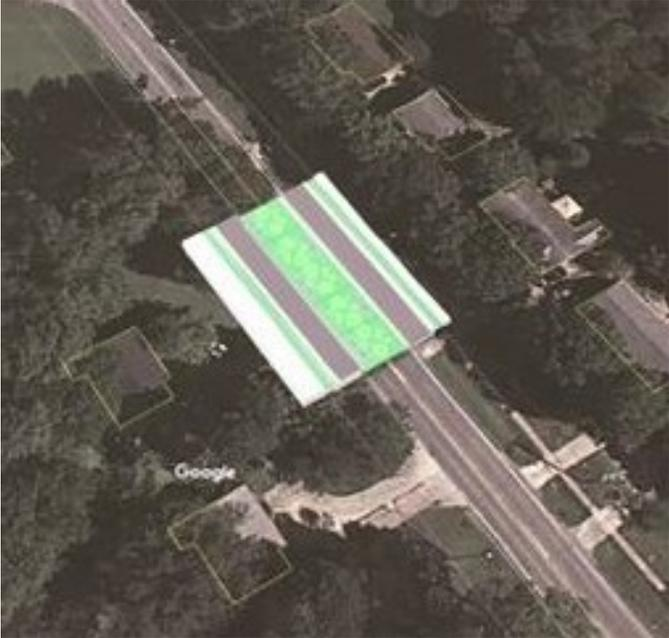
Group 1's plan for this section had a 5' sidewalk on the north, a 10' MUP on the south, and 4' planting strips on both sides of the street. They had an 11' travel lane in each direction separated by a 23' planted median.
